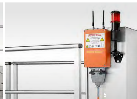
5 Using the remote control, both the semi-automatic as well as the fully-automatic ground sludge remover are easy to operate.
